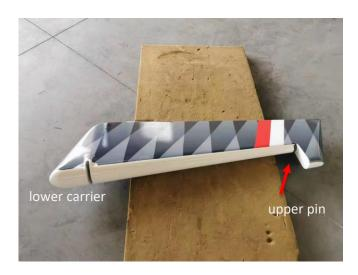
Push the pedals to deflect the VT rudder either to the left or right. Keeping deflected position, insert the VT rudder (its upper pin) into its upper hinge on the tail fin and push its lower carrier to the tail fin at the same time:
