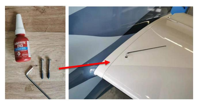
⇒ Prepare two nuts and two washers for M6 screws. Install them on M6 screw fixing the elevator to the steering lever. Install it the same way on the second half of the horizontal tailplane:
