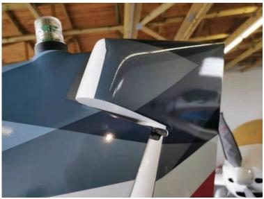
⇒ Prepare two M5x35 stainless screws. Adjust the steering back to neutral position and install both screws on each side of the VT rudder. These fix the VT rudder in the lower carrier:
