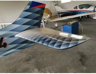
⇒ Install two M8 screws, which connect both halves of the HT, into appropriate holes and screw them into the bulkhead inside the tail. The screws must be secured by the Loctite 243, fitted with a locking washer to avoid their self-loosening and must be properly tightened:
