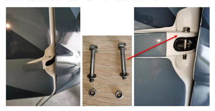
⇒ Install the cover of the mounting hole situated below the left horizontal tailplane:
