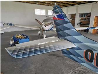
⇒ Connect the left half of the HT same way. At the same time, it is necessary to get the trim servo wire through the hole into the fuselage:
