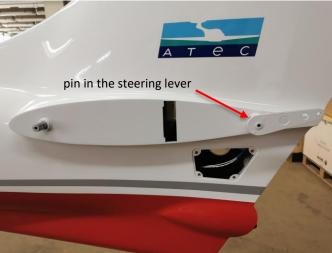
⇒ Connect the right half of the HT with the elevator first. Insert its crossbeam into the hole in the fuselage and insert the elevator into the pins in the steering lever at the same time:
