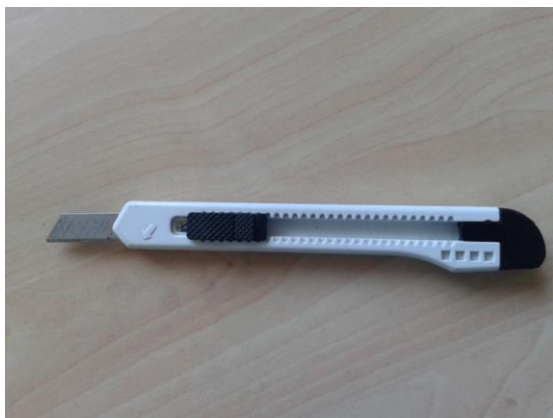
Pic. 1: example of the tool suitable for inspection of coating attachment
