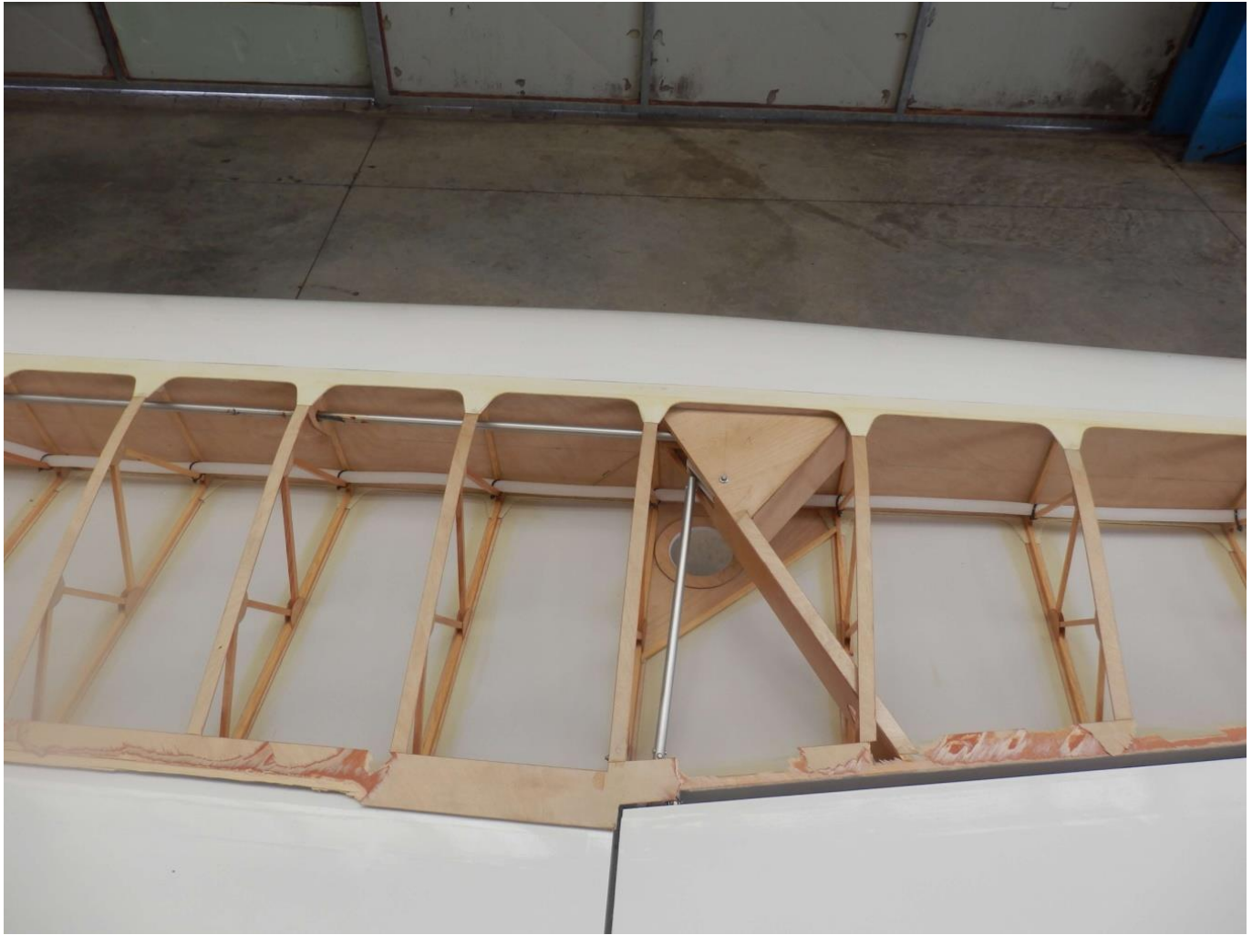
Pic. 3: Fabric coating separated from the upper part of the right wing
