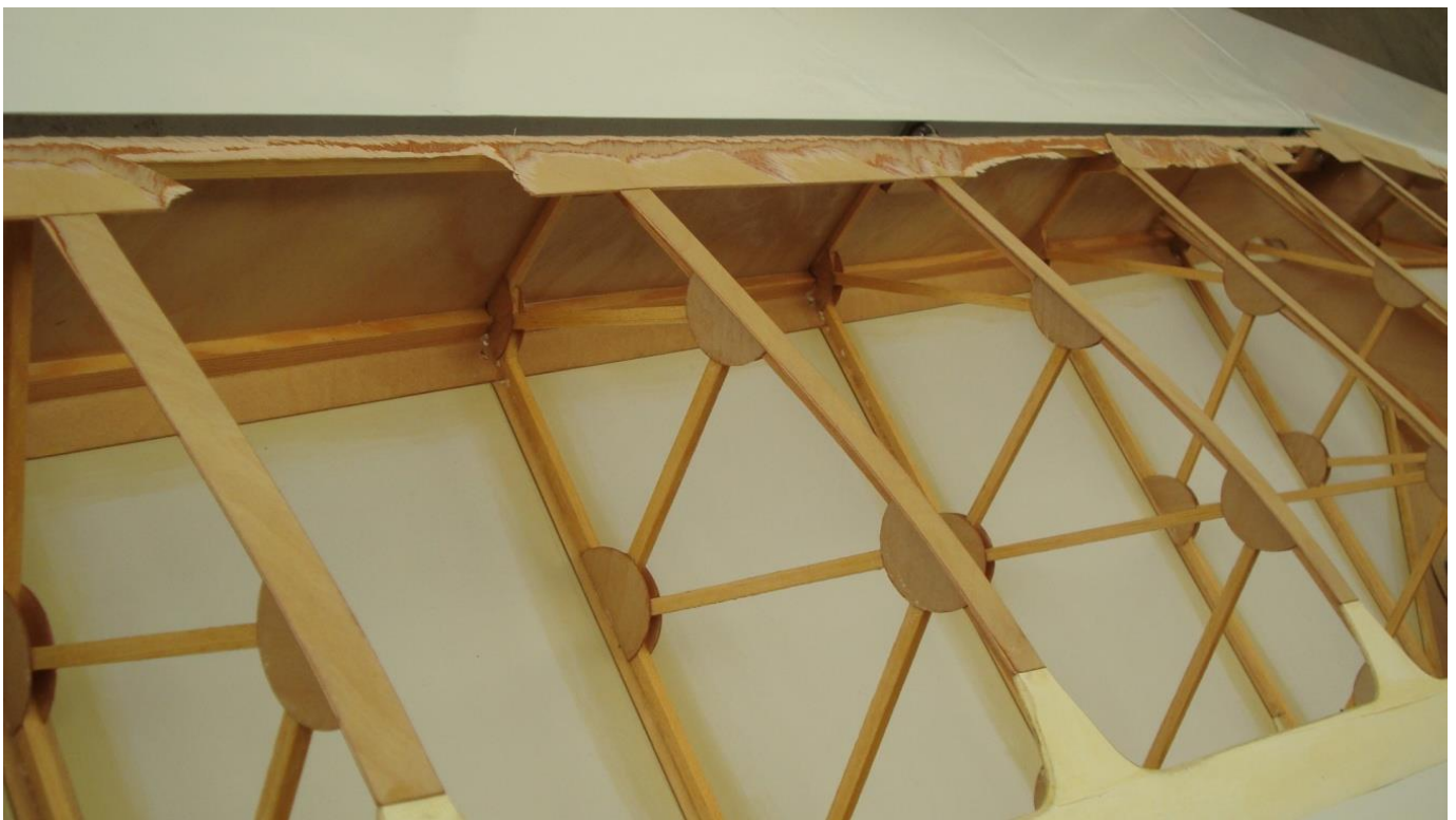
Pic. 2: Fabric coating separated from the upper part of the wing
