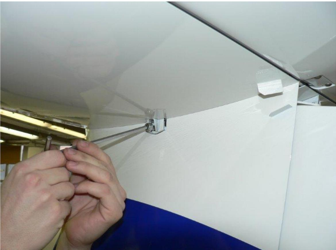
Insert the vertical screw M6 (with nylon) into the hole on the upper side of the HT and tighten it fully with adequate power.
