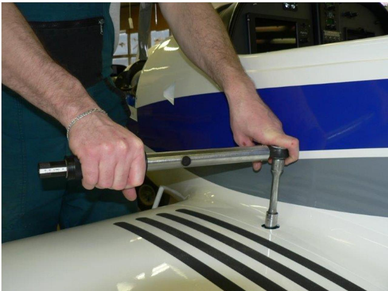
Install the M10 locking nut from the bottom side, so that the wing connection is properly secured.
