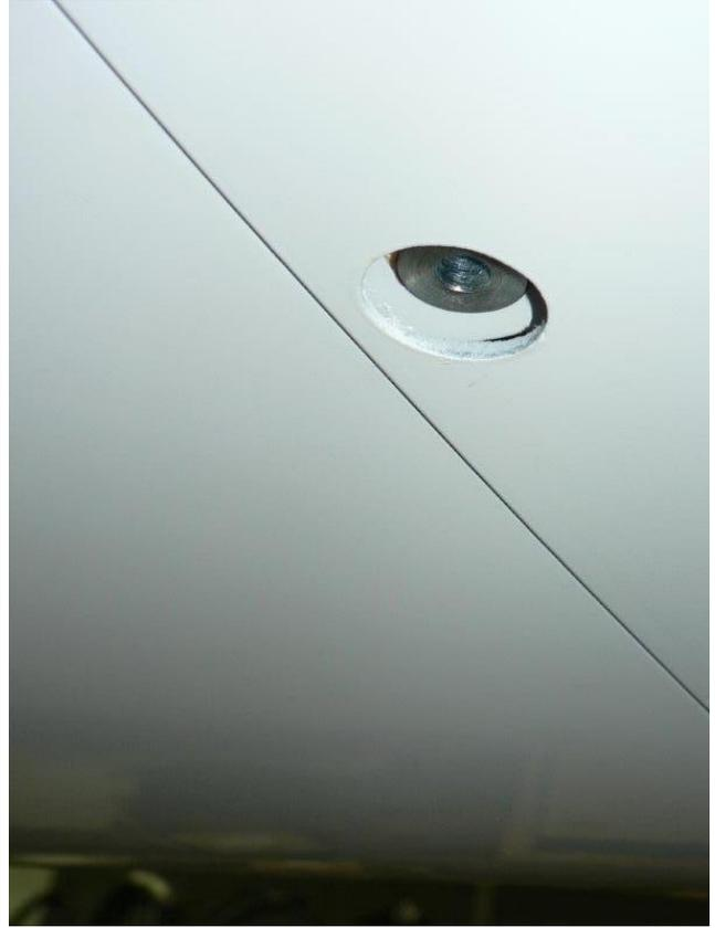
Secure the pin from upper side by the bolt – tightening moment is approx. 25 Nm.
