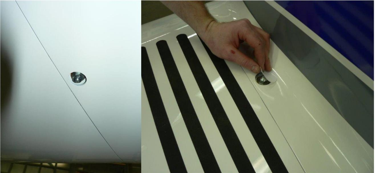
• **Flap pushrods connection inside the cockpit**
