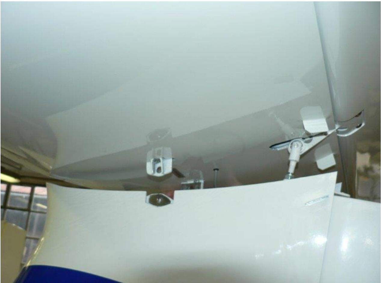
Connect the pushrod with the elevator control lever by the pin of  $\varnothing 5\text{mm}$  and spacer + split pin.
