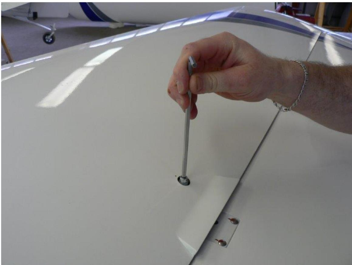
Come back to both main fitting screws M8 and tighten them fully.
