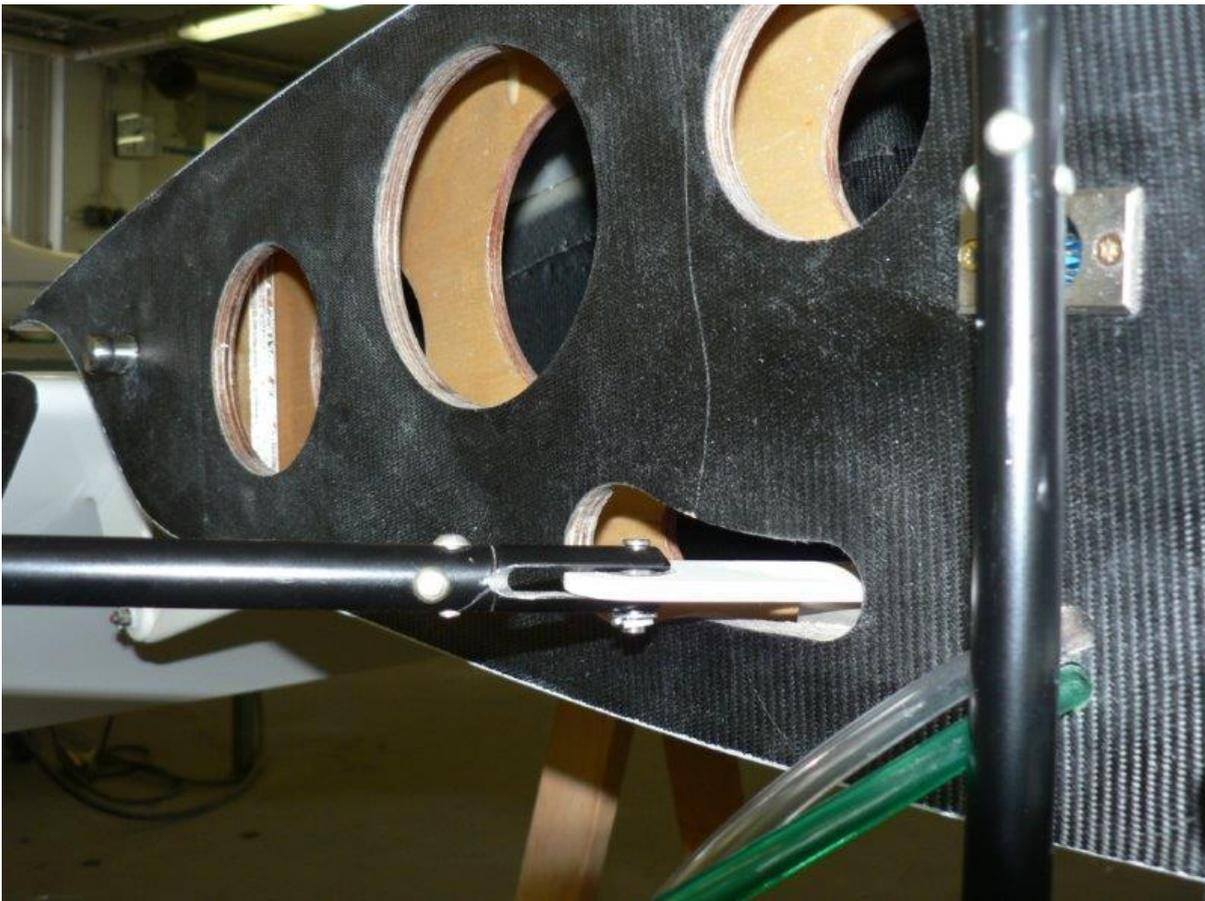
● **Aileron pushrod preparation - connection into the wing**
