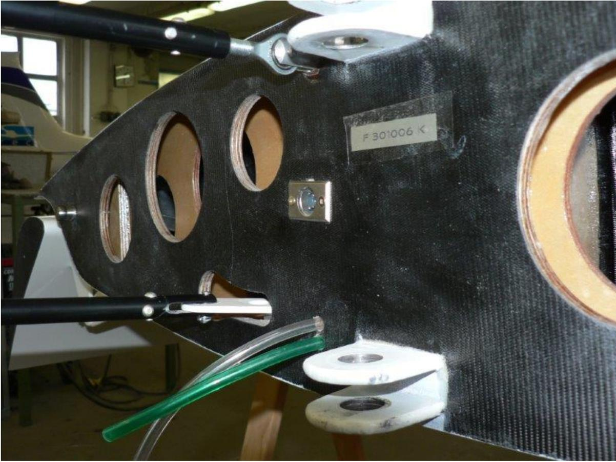
● **Wing connection to the fuselage**
