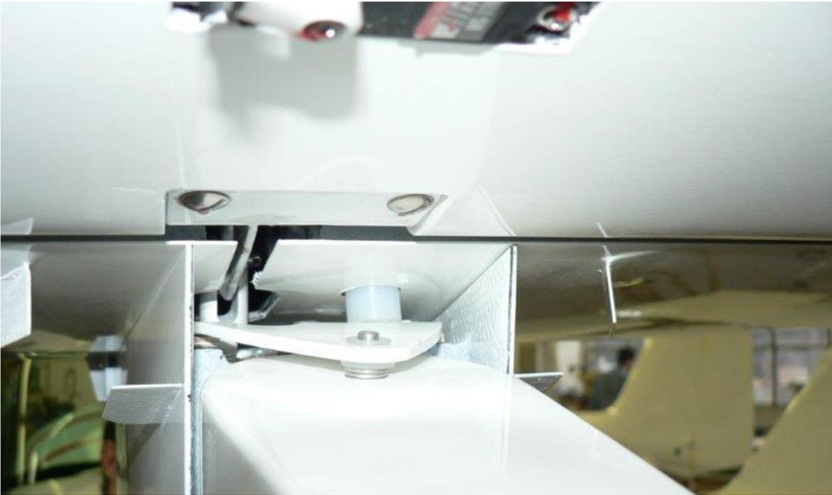
• **Fixing the HT to the fuselage**
