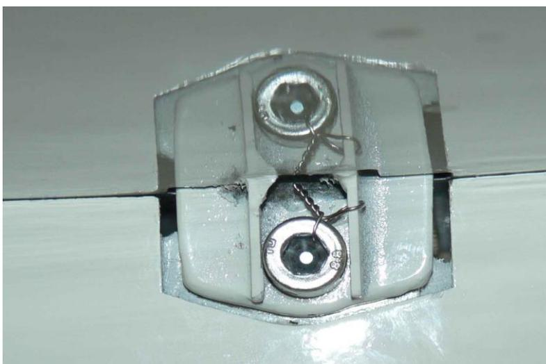
Secure the vertical nylon-screw with a binding wire too. One hole is drilled in the horizontal tail body and two holes are in the screw head.
