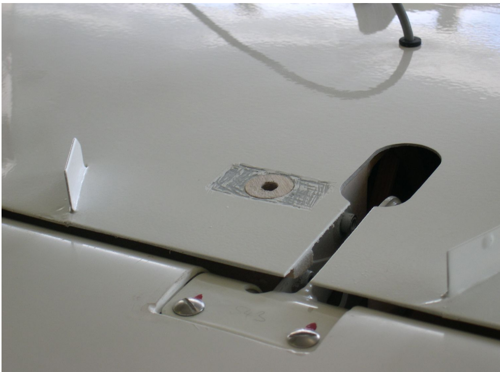
Step 4. - glueing the wooden ring into the hole
